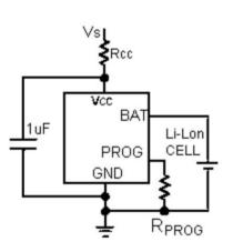
Figure 3: A circuit to increase charging current in thermal regulation mode
