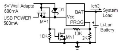
Figure 5: AC adapter and USB power supply combination
