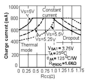
Figure 4: Charging current vs. Rcc relationship curve
