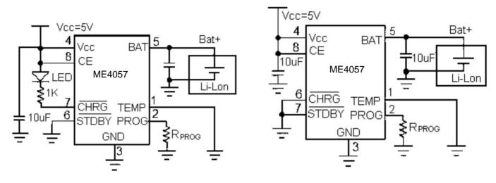
5. Add a power resistor to the input end to reduce chip power loss. When the red light is on, it means it is charging, and when the green light is on, it means the charging is stopped.
