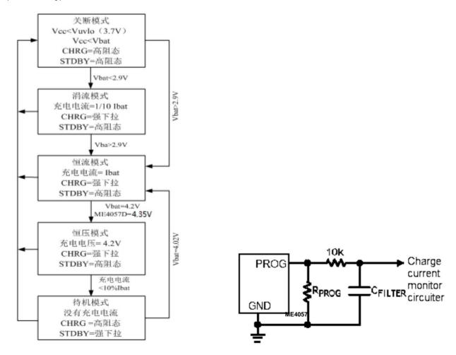
Figure 1: A typical charging cycle status diagram
